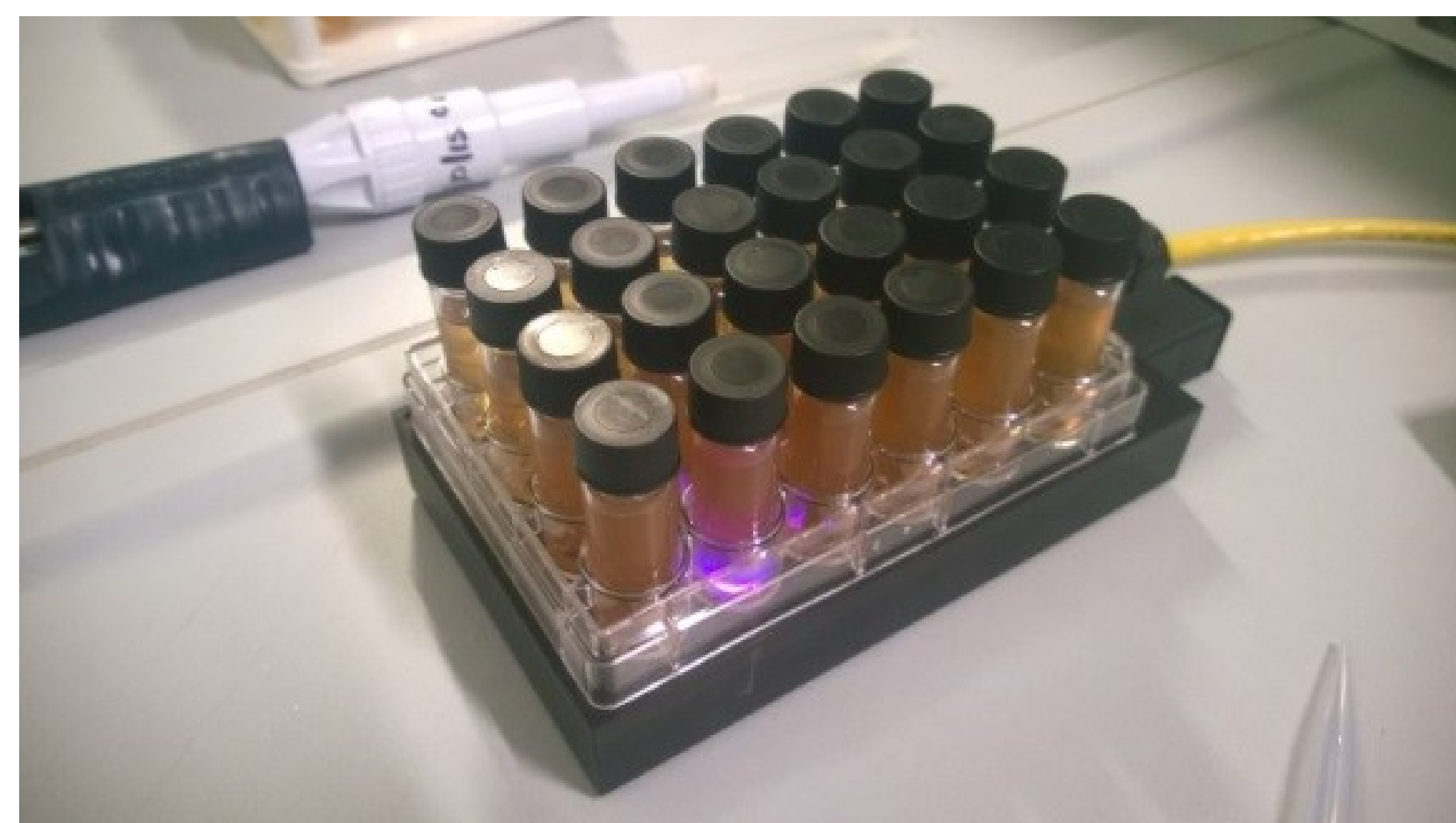
Sensor dish reader used for the study of must oxygen consumption
