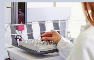
Autosampler performs liquid-liquid extraction immediately prior to injection into GCMS
