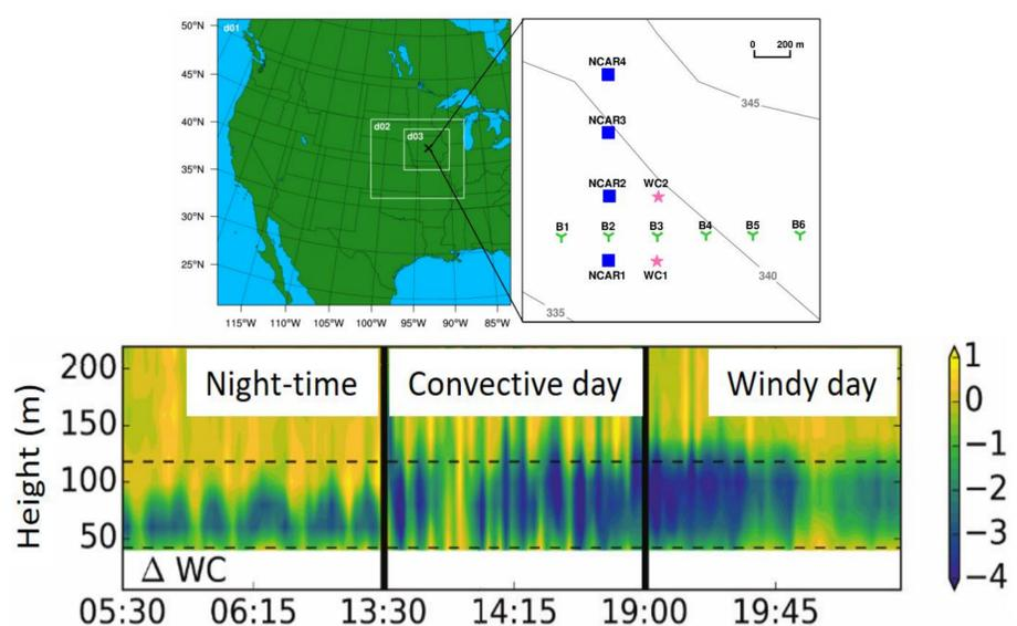
**Figure 2.** Difference in wind speed against time, height and atmospheric condition between an upwind (WC1) and downwind (WC2) region of a wind farm as measured by a Light Detection and Ranging wind profiler. Negative (blue colours) show periods of wind speed reductions due to the operation of the wind farm (adapted from Vollmer et al. 2017)
