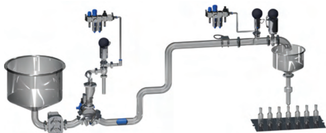
Figure 17. Illustration of a pigging system (Hygienic Pigging Solutions, supplied)
