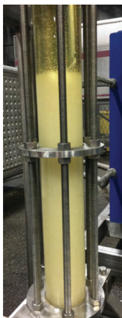
Figure 3. Beginning operation of a fluidised bed crystalliser for wine treatment at pilot scale
