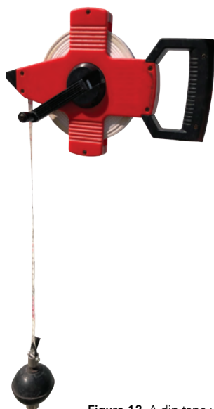
Figure 12. A dip tape used for level measurement. Photo credit: AWRI
